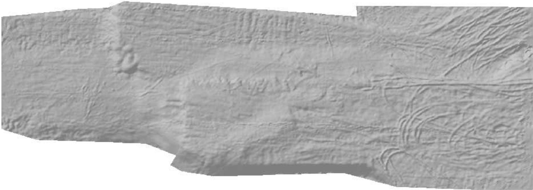
The surface faithfully represents a fine structure on the harbour floor such as remains from the dredge process.
