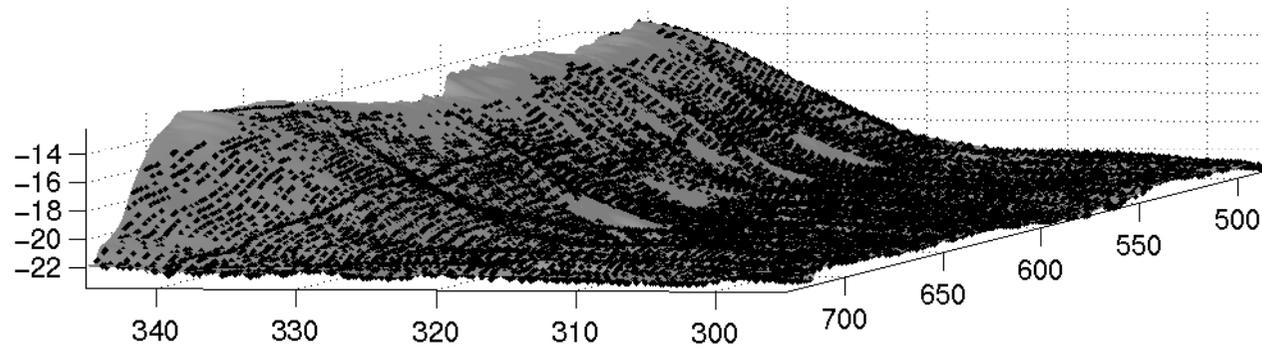
**3) The final spline surface** (142,027 degrees of freedom, 114.6 s computational time, rms error  $< 0.08$  m w.r.t. the cleaned data):
