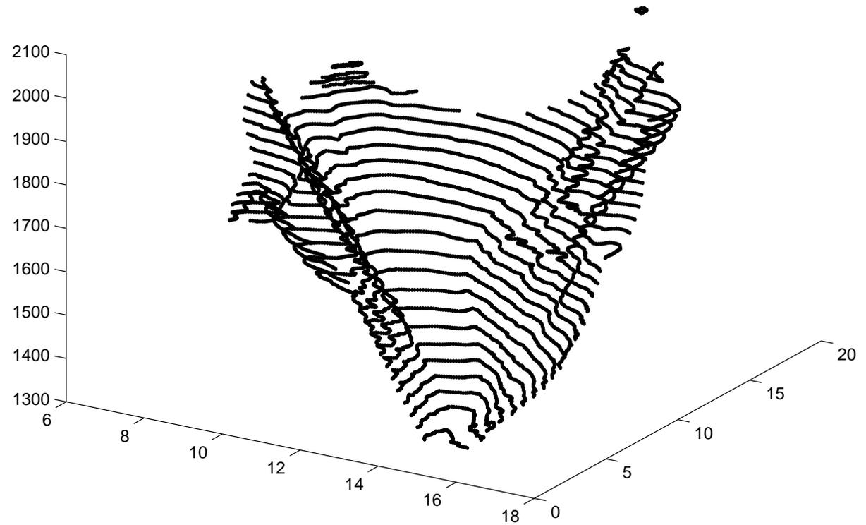
Glacier test: The  $C^2$  spline approximation ( $n_x = 20, n_y = 24$ ) with  $(H_{MQ})$ .
