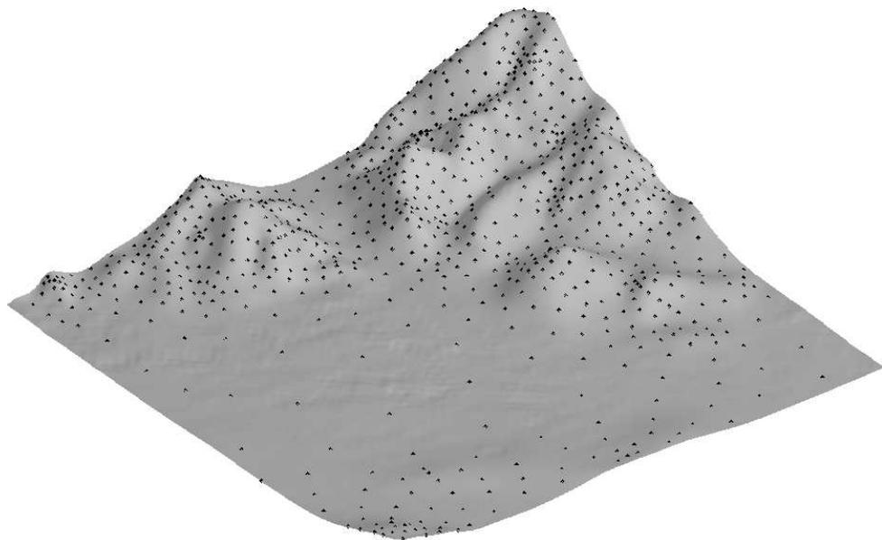
**6. Rotterdam Port multibeam echosounder data** 634,604 raw data points (courtesy Quality Positioning Services, Zeist, Holland).
