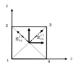
Figure 4: Redefined Face-Based Shape Functions.
